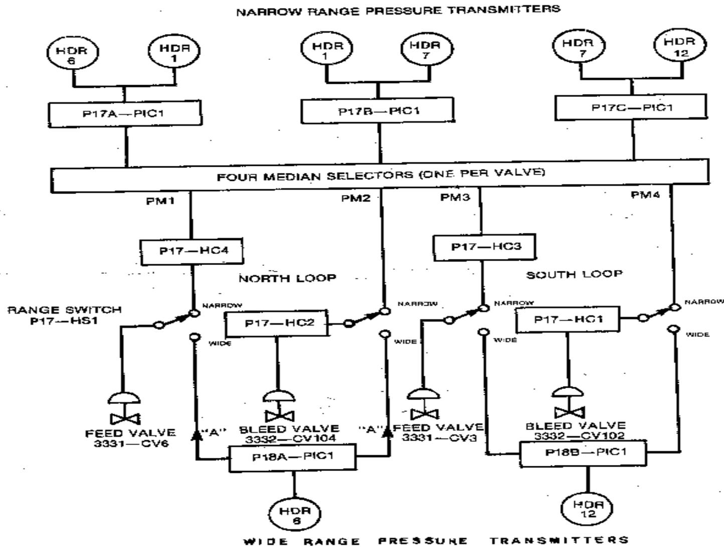
Figure 3: Heat Transport Pressure Control Scheme.
