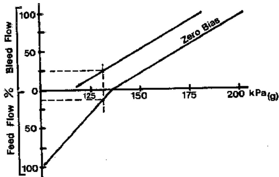
Figure 4: Feed and Bleed Flows vs Control Signal.
