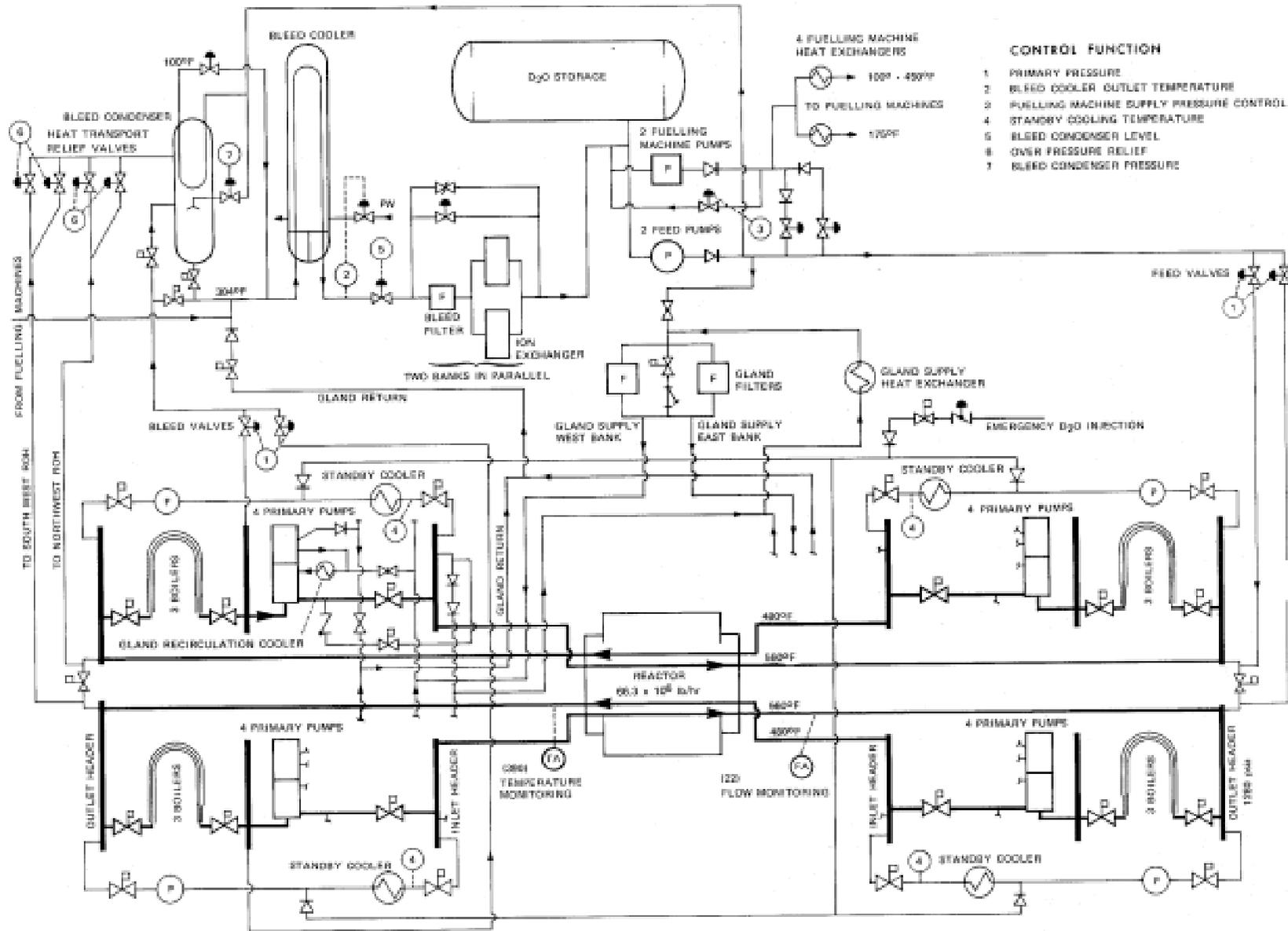
Figure 1: 500 MWe CANDU Heat Transport System with Feed and Bleed Pressure Control.
