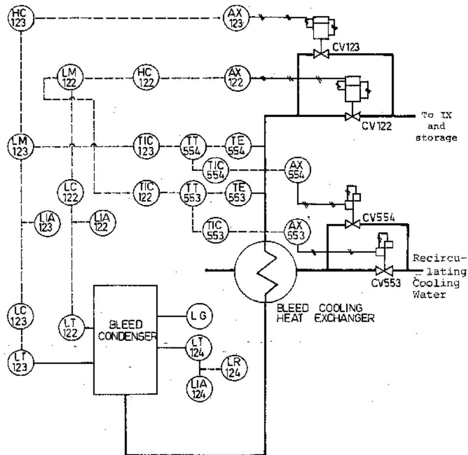
Figure 2: Bleed Condenser Level and Bleed Temperature Control.
