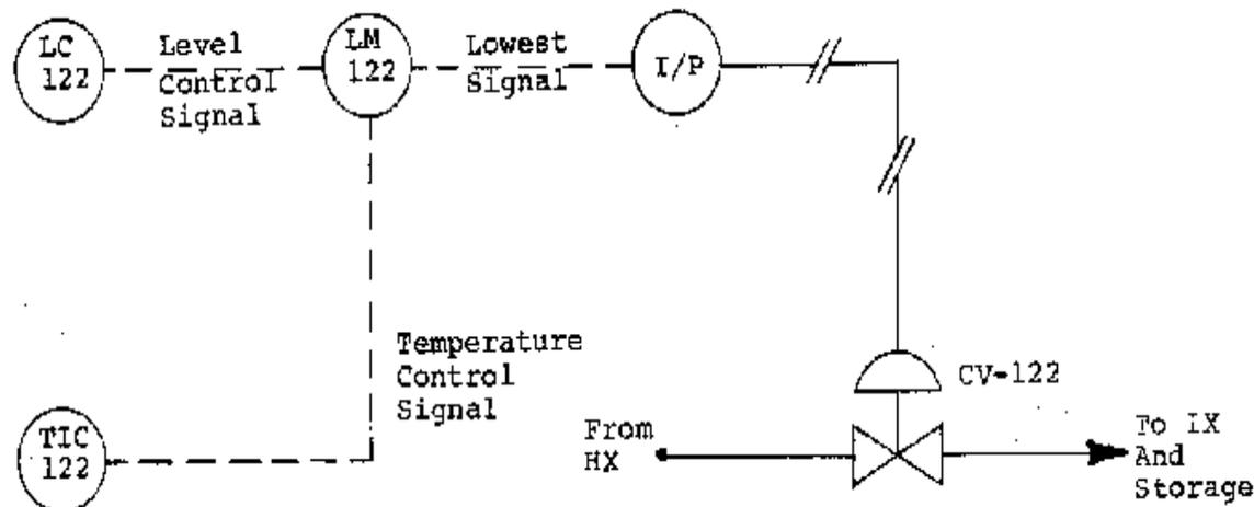
Figure 4: Interconnection of the Level and Temperature Controllers.
