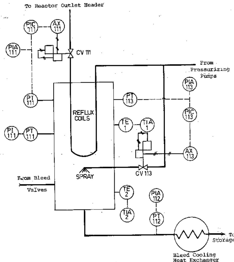
Figure 1: Bleed Condenser Pressure Control.
